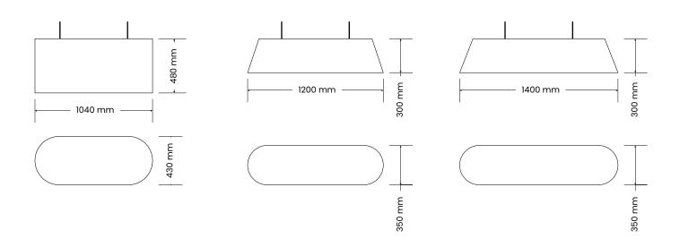
All dimensions can be customised to specification and can be manufactured with vertical or tapered sides
