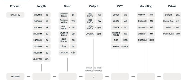
Note the Linear 90 can be manufactured with direct light only or with direct & in-direct light. If only direct light is required, specify the direct wattage only. The standard in-direct wattage is 7W.
