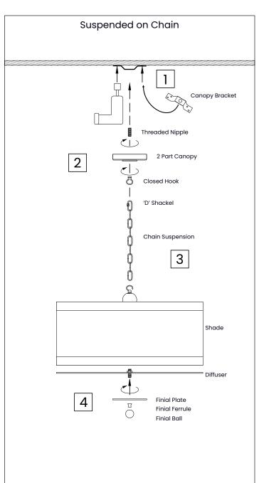
1 Attach the canopy bracket to the ceiling
